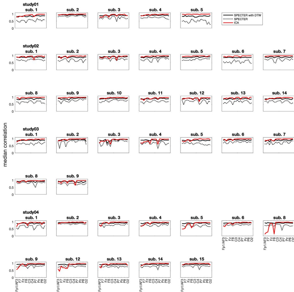
Fig. 12. Dataset 2: The median Spearman’s correlation coefficient between the original EEG signal and EEG signal reconstructed by SPECTER and ICA (red line) over rest epochs. In the case of SPECTER, the correlations were computed using only the SPECTER algorithm (black dotted line) or SPECTER followed by heuristics described in Section 2.1 and the DTW algorithm for solving the slight time shift and opposite sign problem (black line). Only labels for each second electrode are depicted on the x-axes.
